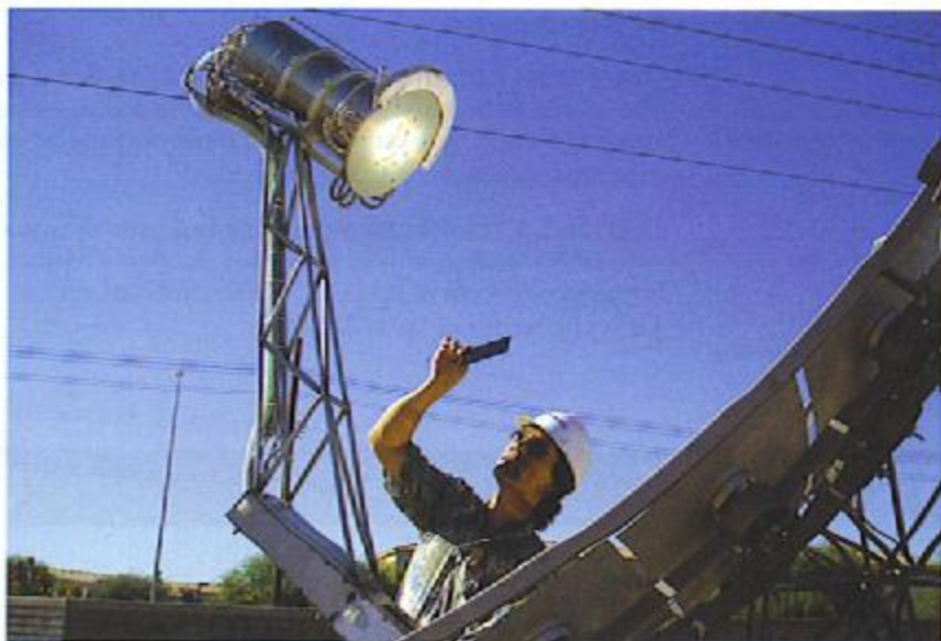
Above: SHEC Labs' solar hydrogen generator uses concentrated sunlight at 5,000 times the intensity of the sun in its thermochemical hydrogen production process.
